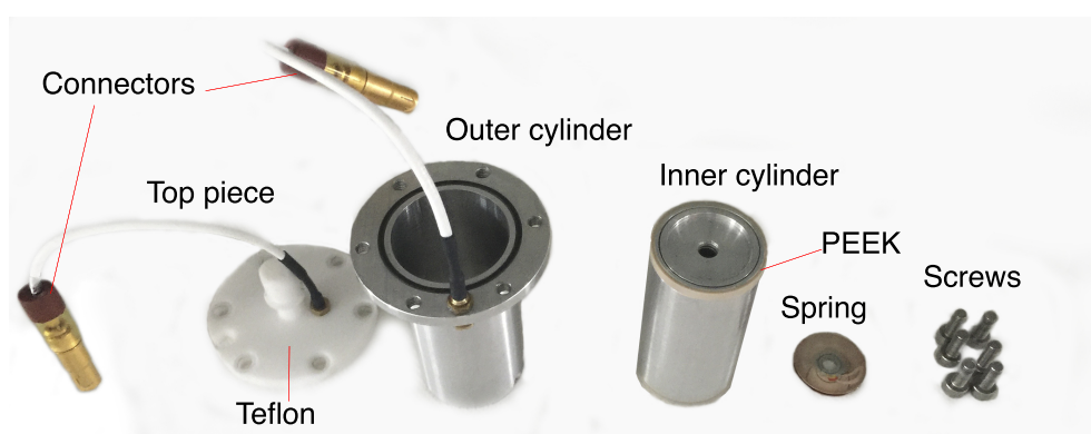
Figure C.3: a picture of the completely disassembled cell used in 2016.
