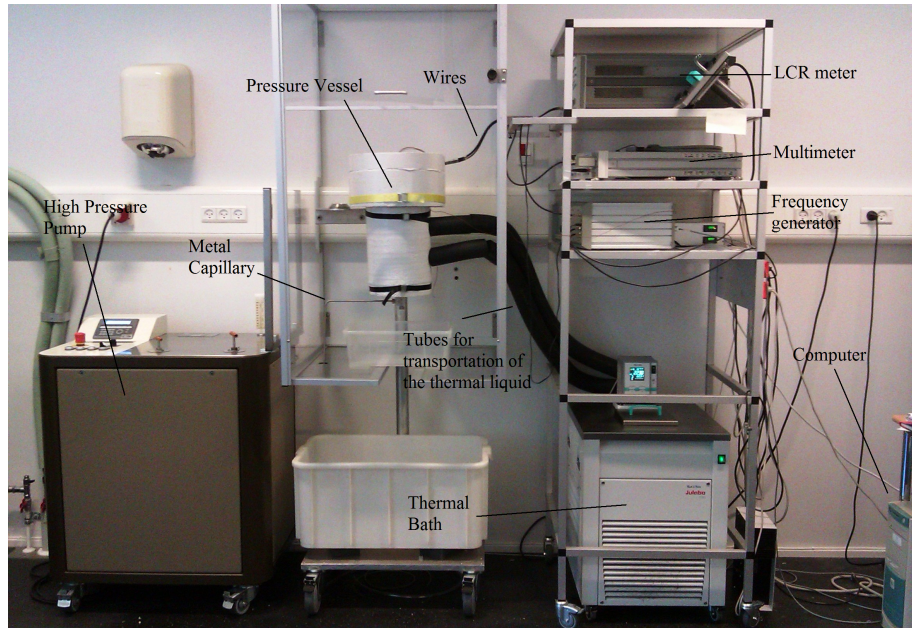
Figure 4.2: The pressure setup. Picture from Roed (2012) [59].
