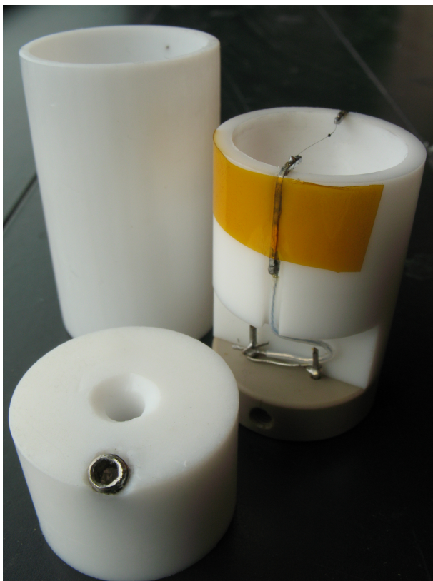
Figure B.1 Photo of the three parts constituting the moulding device. See the text above for an explanation.
