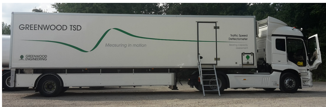
FIGURE 4.3: The Traffic Speed Deflectometer vehicle used in this study. Strain gauges are mounted on the rear-end axle.
